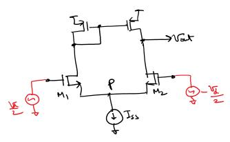
Circuit is not symmetric Ideally P is not the ground in differential picture
