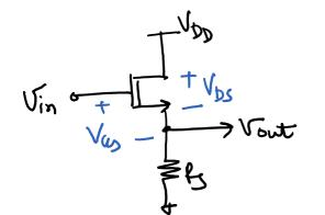
$$V_{DS} = V_{DD} - V_{avt}$$
