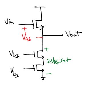
Issue with SF as a better DC level shift I limited input swing VOD Vin Vin > Vas + 2Vos, sat Ъ
