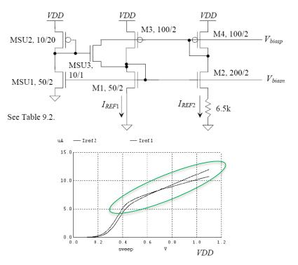
Figure 20.18 Beta-multiplier reference for short-channel design (see Table 9.2).
