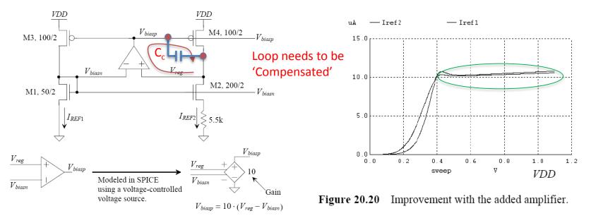
Figure 20.19 Increasing the output resistance of short-channel MOSFETs using feedback. The result, for the Beta-multiplier circuit, is better power supply sensitivity.
