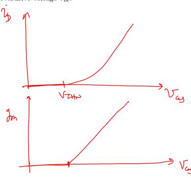
(b) (5 points) Sketch  $g_m$  as a function of current  $(I_D)$  when the W/L ratio is constant.
