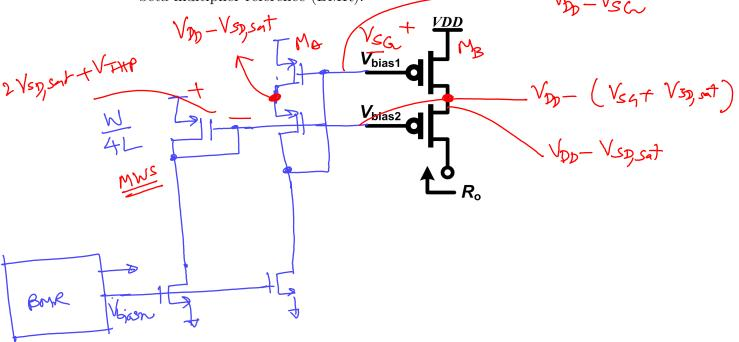
(b) (5 points) Derive an exact expression for the output resistance of the cascode current source seen above.
