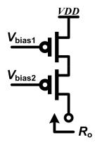
(b) (5 points) Derive an exact expression for the output resistance of the cascode current source seen above.
