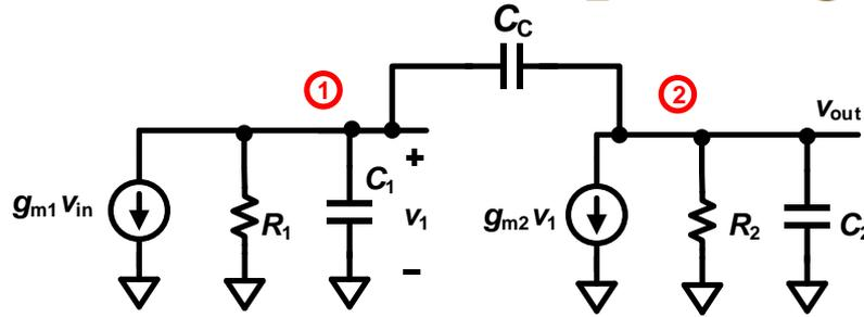
$$\frac{v_{out}}{v_{in}}(s) = \frac{A_v \left(1 - \frac{s}{\omega_z}\right)}{\left(\frac{s}{\omega_{p1}} + 1\right) \left(\frac{s}{\omega_{p2}} + 1\right)}$$
