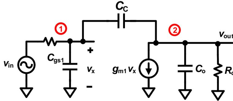
$$\frac{v_x - v_{in}}{R_s} + v_x s C_{gs1} + (v_x - v_{out}) s C_{gd1} = 0 \quad (1)$$
