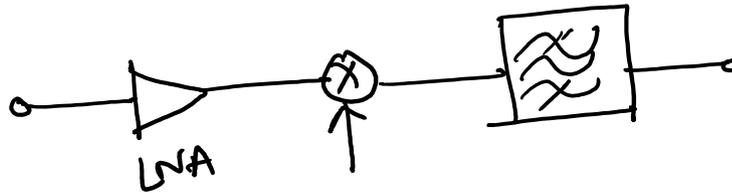
Need to calculate: the noise factor (figure) of the entire Rx chain as a function of  $F$  and gain of the individual blocks in the Rx chain.
