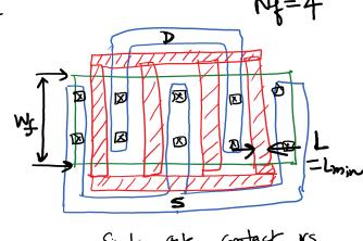
Single gate contact vs double gate contact + Pg is reduced with Read from Chipter 4 MOSFET Section
