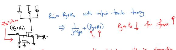
Need Real impedance at the input without degrading NF or BW.
