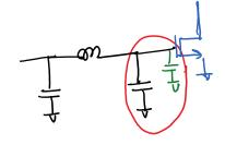
Janusite capacitance can be absorbed in the network design. T- Match.
