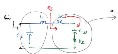
$\Rightarrow Q \text{ of the right hand 1-section}$   $\Rightarrow Q \text{ right} = \frac{\omega_0 L_2}{R_{\pm}} = \sqrt{\frac{R_F}{R_{\pm}} - 1}$
