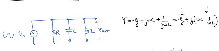
$$Y = -g + j\omega C + \frac{1}{j\omega L} = -g + j(\omega C - \frac{1}{\omega L})$$
