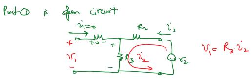
$$Z_{21} = \frac{V_2}{v_1} = R_3$$
