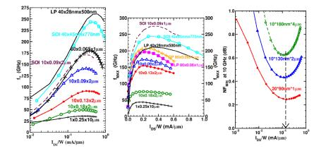
J<sub>pfT</sub> = where f<sub>T</sub> reaches its max (NMOS= 0.3 - 0.4 mA/μm)
