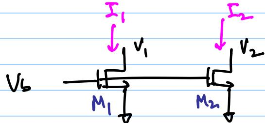
$$I_D = \frac{\mu n C_{ox}}{2} \frac{W}{L} (V_{DS} - V_{THN})^2 (1 + \lambda V_{DS})$$
