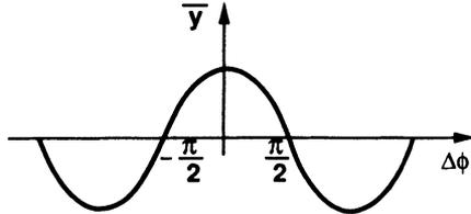
Fig. 10 Characteristic of a sinusoidal PD.
