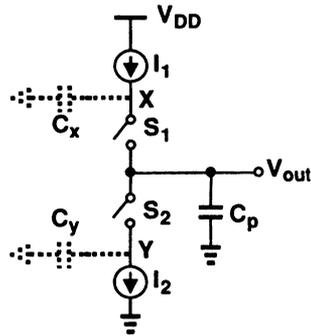
Fig. 50 Charge-sharing in a charge pump.
