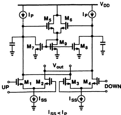
Fig. 51 Differential CMOS charge pump.
