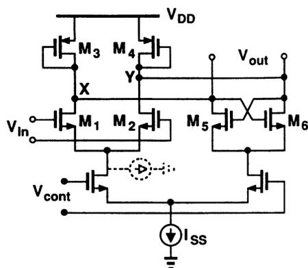
Fig. 34 Delay variation using local positive feedback.
