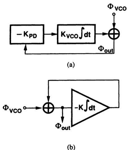
Fig. 57 Simplified model of PLL with VCO noise.
