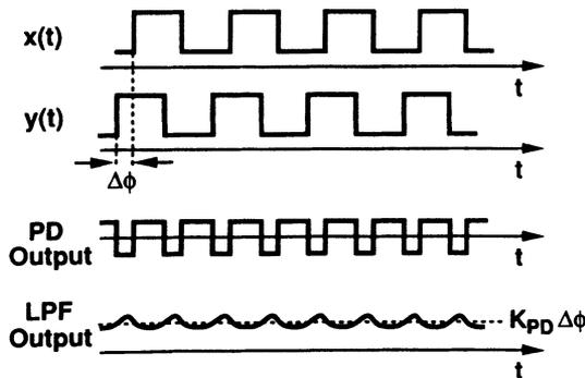
Fig. 12 Waveforms in a PLL.
