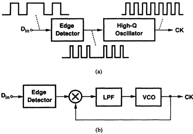
Fig. 62 (a) Conceptual realization of a CRC; (b) phase-locked CRC.
