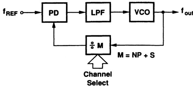
Fig. 70 Phase-locked synthesizer.
