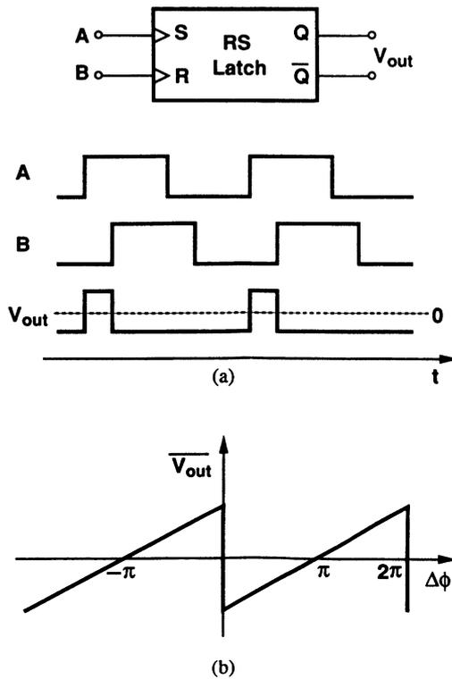
Fig. 40 Edge-triggered R-S latch as a PD.
