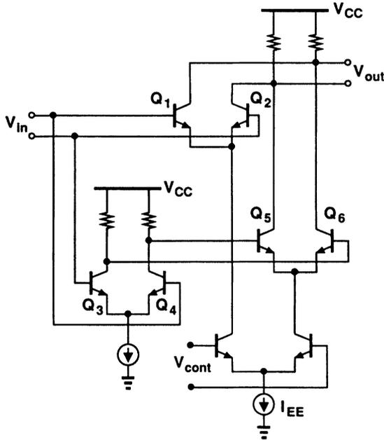
Fig. 31 Delay interpolation in a bipolar VCO.
