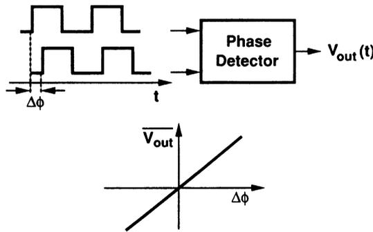
Fig. 8 Characteristic of an ideal phase detector.
