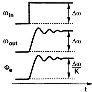
Fig. 16 Response of a PLL to a frequency step.
