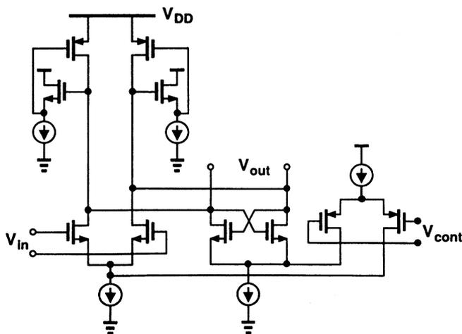
Fig. 35 Low-voltage variable-delay gain stage.
