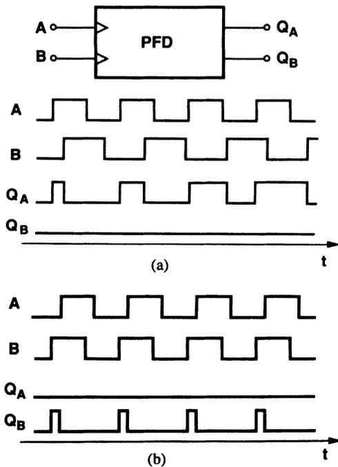
Fig. 42 Phase/frequency detector response with (a)  $\omega_A < \omega_B$ ; (b)  $A$  lagging  $B$ .
