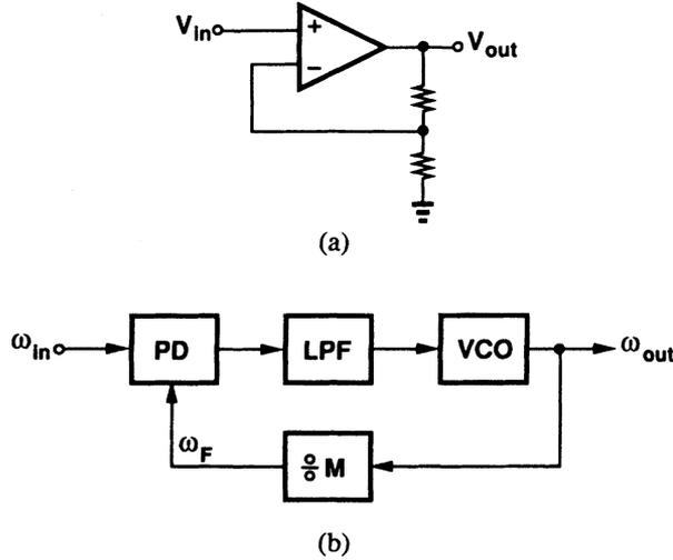
Fig. 26 Signal “amplification” in (a) a feedback amplifier; (b) a PLL.
