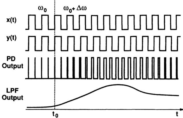
Fig. 13 Response of a PLL to a small frequency step.
