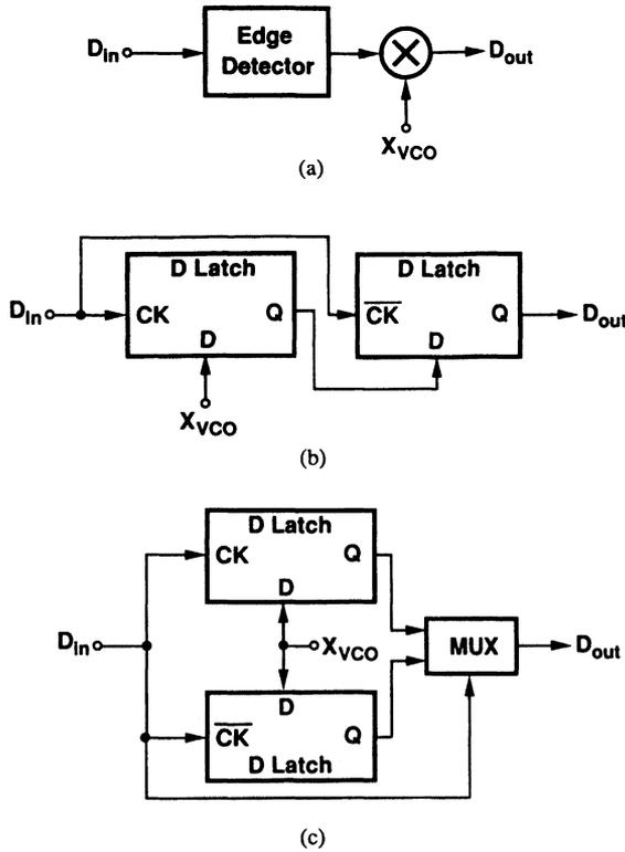
Fig. 61 Edge detection and sampling of NRZ data.
