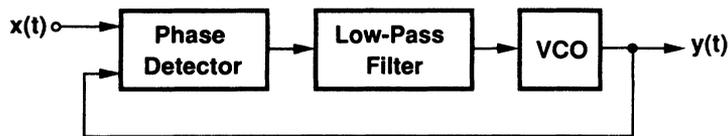
Fig. 11 Basic phase-locked loop.
