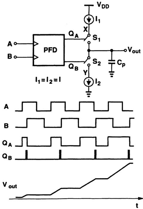
Fig. 47 PFD with charge pump.
