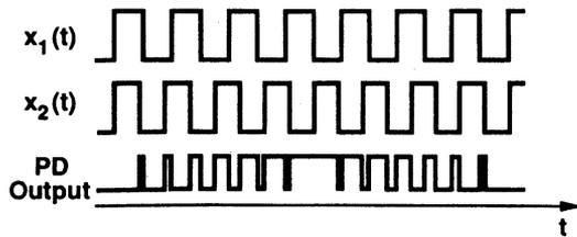
Fig. 9 Input and output waveforms of a PD.
