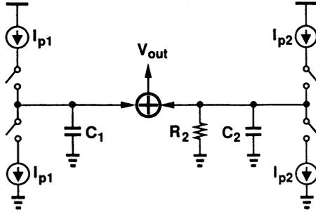
Fig. 54 Addition of zero by means of feedforward.
