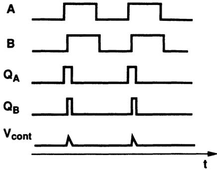
Fig. 49 Effect of mismatch in current sources of a charge pump.
