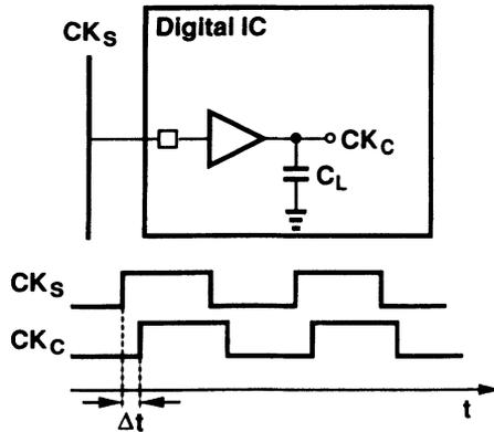
Fig. 2 Clock skew in a digital system.
