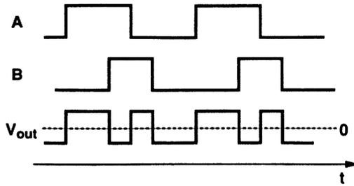
Fig. 39 Dependence of XOR output on input duty cycle.
