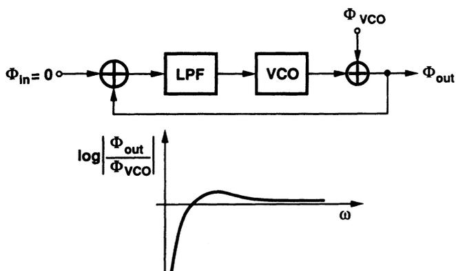
Fig. 56 Noise transfer function of a PLL from VCO to output.
