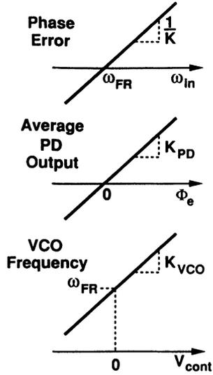
Fig. 19 Variation of parameters during tracking.
