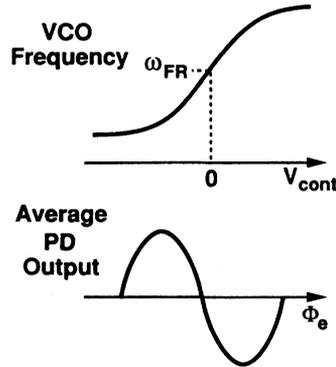
Fig. 20 Gain reduction in PD and VCO.
