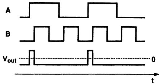
Fig. 41 Response of R-S latch to higher harmonics.
