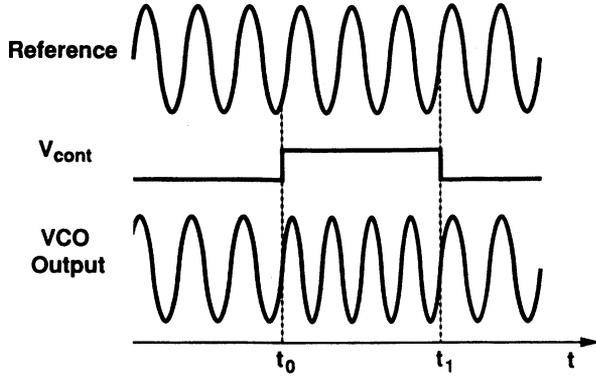
Fig. 7 Phase alignment of a VCO with a reference.
