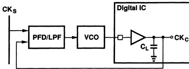
Fig. 69 Skew reduction using a PLL.
