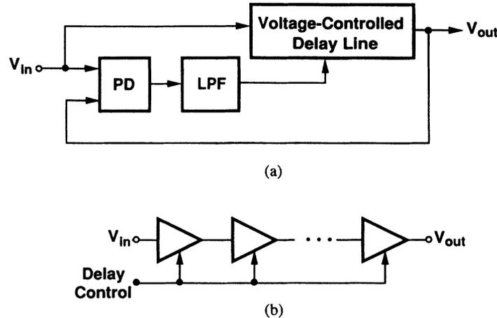
Fig. 27 (a) DLL block diagram; (b) delay line.
