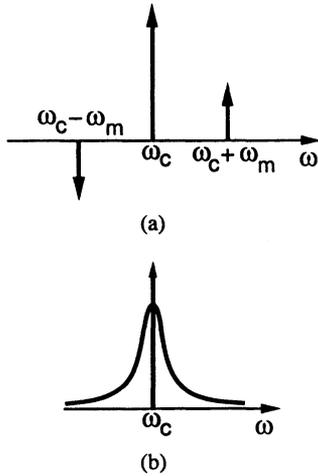
Fig. 5 (a) Sidebands and (b) noise skirts resulting from phase modulation.
