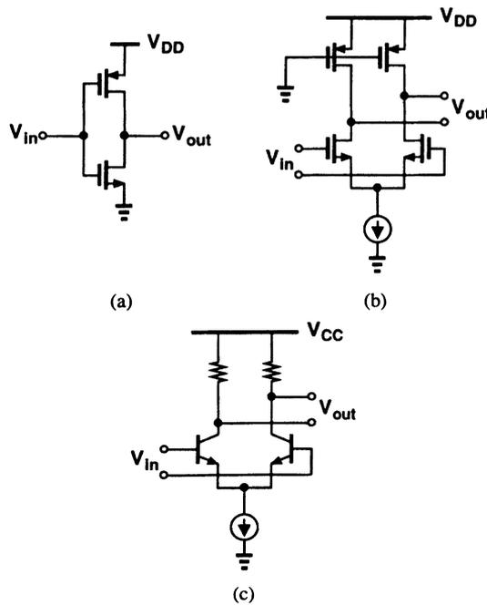
Fig. 29 Simple gain stages.
