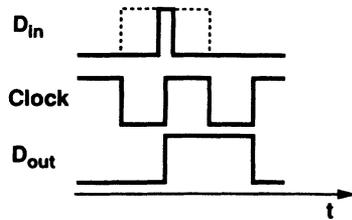
Fig. 68 Jitter margin for correct sampling of data.
