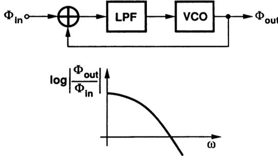
Fig. 55 Noise transfer function of a PLL from input to output.
