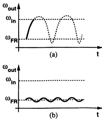
Fig. 23 (a) Capture with no cycle slips; (b) capture failure.
