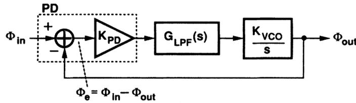
Fig. 14 Linear model of a PLL.
