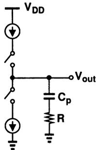
Fig. 53 Addition of a zero to a charge pump.
