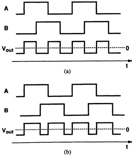
Fig. 37 Input and output waveforms of an XOR gate.
