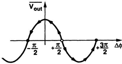
Fig. 18 Phase variation to provide negative feedback.
