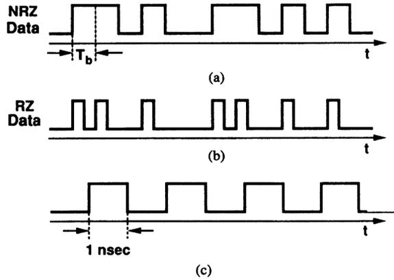
Fig. 58 (a) NRZ data; (b) RZ data; (c) fastest NRZ waveform with  $r_b = 1 \text{ Gb/s}$ .
