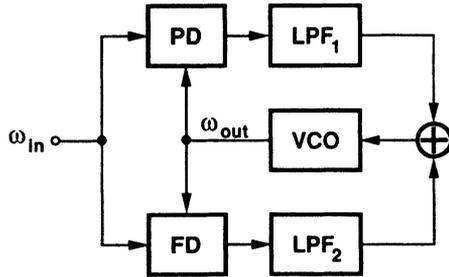
Fig. 25 Aided acquisition with a frequency detector.
