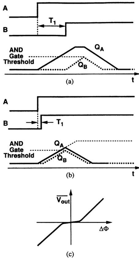
Fig. 48 Dead zone in a PFD with charge pump.
