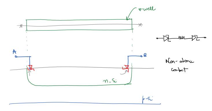
A Metal in intact with moderately or lightly defeal Si froms a metal-semiconductor disde (schattley disde).
