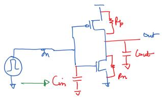
$$C_{in} = \frac{3}{2} \left( C_{OXIN} + C_{OXIP} \right)$$
