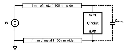
(a) (5 points) How much is the peak supply droop and ground bounce in the circuit?
