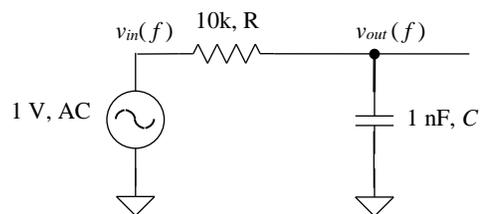
b) Using the equations in part (a), sketch properly labeled Bode magnitude and phase plots.
