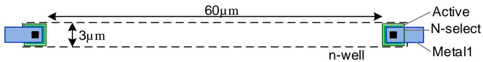
b) If the bottom zero-bias depletion capacitance of the n-well to substrate is  $100 \text{ aF}/\mu\text{m}^2$  (a is atto or  $10^{-18}$ ), the sidewall capacitance is  $50 \text{ aF}/\mu\text{m}$ , then estimate the delay through the resistor.
