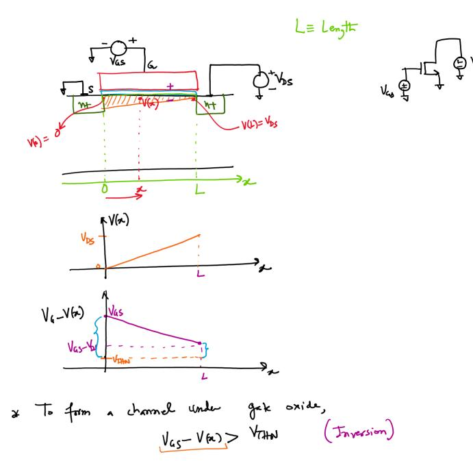
the donsity of electrons in the channel follows the trend of Vas-V(x), and falls to a minimum at x=L
