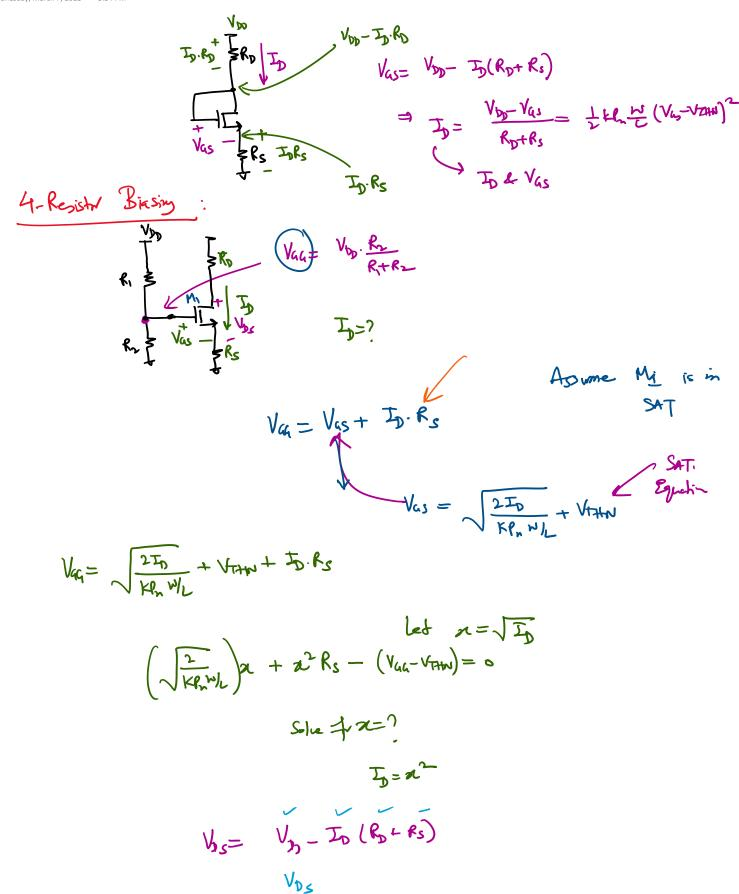
check for saturation  $V_{Ds} = V_{GS} + V_{THN}$
