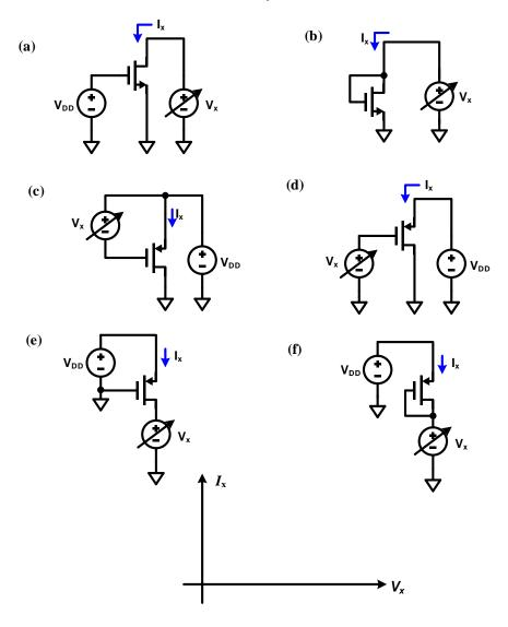
3) Using Cadence, generate all I-V curves (i.e.  $I_D$ - $V_{GS}$  and  $I_D$ - $V_{DS}$  for varying  $V_{GS}$ ) for NMOS and PMOS of sizes  $18\mu/0.18\,\mu$  and  $36\,\mu/0.18\,\mu$  respectively. Find  $V_{THN}\,(V_{THP})$  and  $V_{DS,sat}$  ( $V_{SD,sat}$ ) for both NMOS (and PMOS). Label the plot along with the cutoff, triode and saturation regions.
