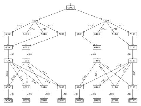
FIGURE 12. Model  $\mathcal{M}_1(\text{Ring}, n, 1)$ . The components of the state are position, value, extrema[0], extrema[1]. For process 0 (top),  $c = c_0$  and  $d = c_{n-1}$ . For process i ( $1 \le i \le n-2$ , bottom),  $c = c_i$ ,  $d = c_{i-1}$ . Process n-1 is not shown, but is like process i with the last transition removed.
