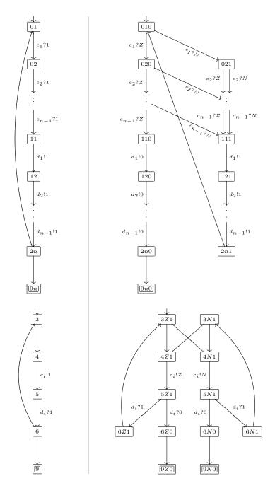
FIGURE 14. Models  $\mathcal{M}_0(\operatorname{Noexit}, n)$  (left) and  $\mathcal{M}_1(\operatorname{Noexit}, n)$  (right). Channel  $d_i$  sends from process 0 (top) to process i (bottom,  $1 \leq i \leq n-1$ );  $c_i$  from i to 0. The first component of the state vector is position. The additional components are i (upper left); i, sbuf[0] (upper right); and sbuf[0], rbuf[0] (lower right).
