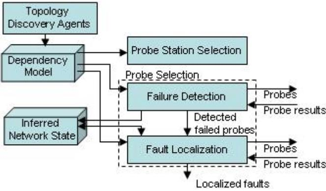
Fig. 1. System architecture for fault diagnosis using adaptive probing.
