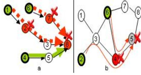
Fig. 2. (a.) 3 independent paths to node 8 from probe station nodes 1, 6, and 4, to detect failure of node 8 in a scenario of failure of 3 nodes (nodes 2, 7, and 8); (b.) A scenario of failure of nodes 4 and 5, where inappropriate probe station placement (at nodes 2 and 6) makes node 5 a shadow node;
