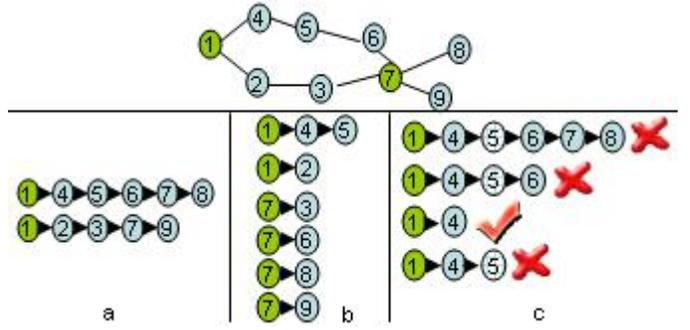
Fig. 3. Network with nodes 1 and 7 as probe stations. (a., b.) Nodes probed by a small set of long probes and larger set of short probes respectively; (c.) Probes sent in a binary search fashion on a failed probe path.
