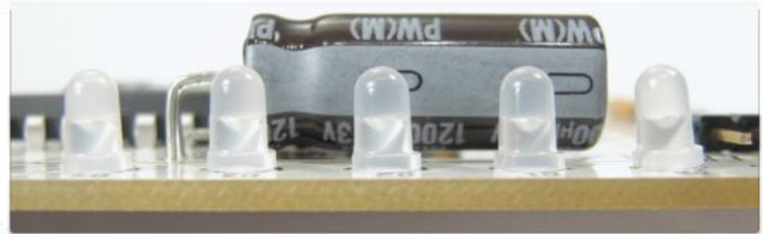
Then push the LEDs flush to the board and solder them in place.
