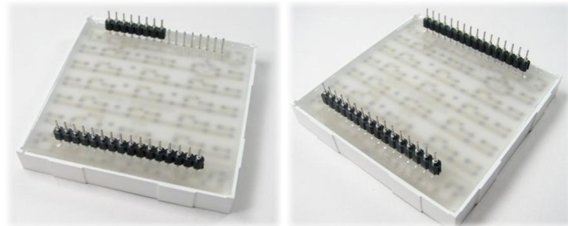
4. Add the other three socket strips to the LED display the same way. This completes the socket assembly; next, we'll add it to the board!
