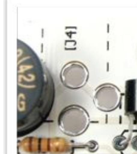
Note: J4 is a location to install a power jack on the reverse side of the board. Your ac adapter should output for 4.5 - 5V dc, regulated, center-positive, with at least 600 mA capacity.
