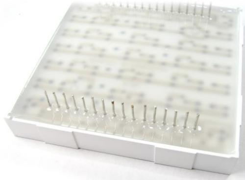
1. Start with the LED matrix display upside down. To avoid scratching the black paint on the front, set it on a clean soft surface like a piece of paper. (*This page will do nicely!*)
