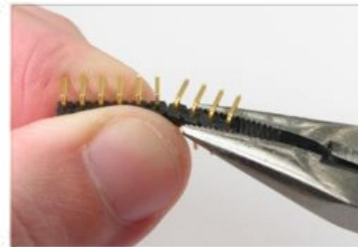
**2.** Holding steady the pins between your fingers, rock the pliers back and forth to split the header in two. It will either split into two parts as 6/4 pins or 7/3 pins. (Either is okay.)
