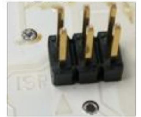
Installed on bottom side (Pin 1 is marked.)
