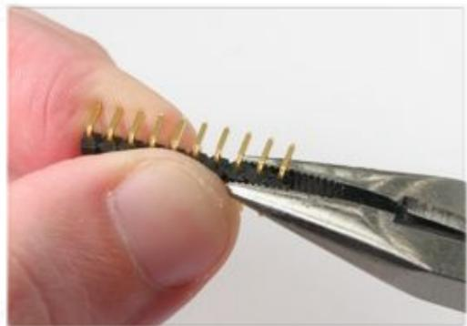
**1.** Using small pliers, grip the first three positions of the header. Hold the rest of the pins-- *tight*-- with your fingers.
