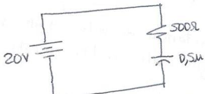
$$\text{Para } t=\infty \quad V_C = 20V \quad \tau = RC = 0,25\text{ ms}$$
