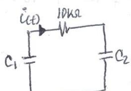
$$I_0 = \frac{V_{C1}(0^+) - V_{C2}(0^+)}{10k\Omega} = \frac{15 - 25}{10k\Omega} = -1mA$$
