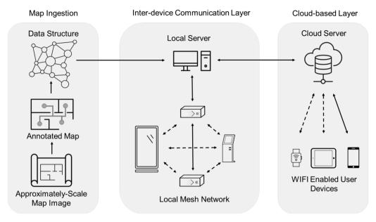
Fig. 4. A diagram showing three layers of the system including map ingestion, inter-device communication, and cloud-based servers. The diagram uses icons of mobile devices, different display units, computers, and data structures to provide an overview of the current and future system using solid and dashed lines.
