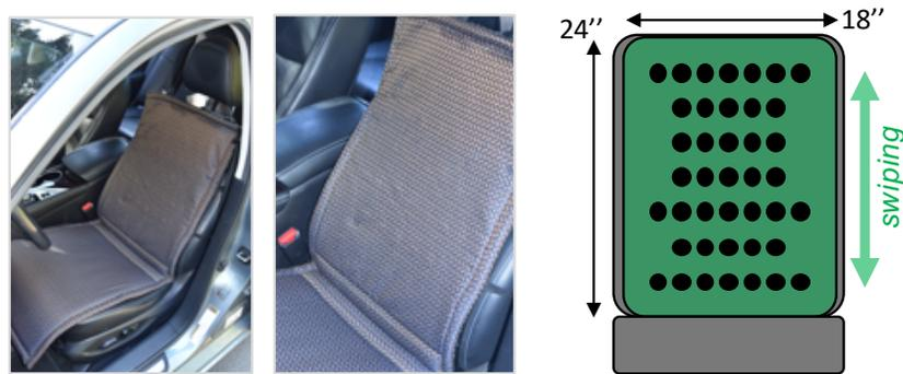
Fig. 2. Seat configuration covering a back space of 12x18 inch grid, able to produce a variety of haptic stimulation patterns.
