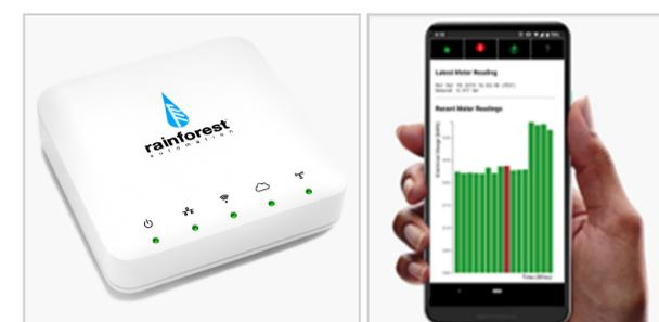
Fig 2: Our prototype system relies on the Rainforest Automation EAGLE-200 home energy hub for access to real-time energy data (left) and we are designing real-time energy displays and learning modules that support the KYEN program's education goals through a collaboration with the METER team at The University of Oxford (right).
