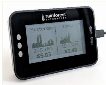
**Figure 1:** A Rainforest Automation™ EMU-2 device illustrates one type of energy display that families could use to assist them with understanding energy use and pricing at home.
