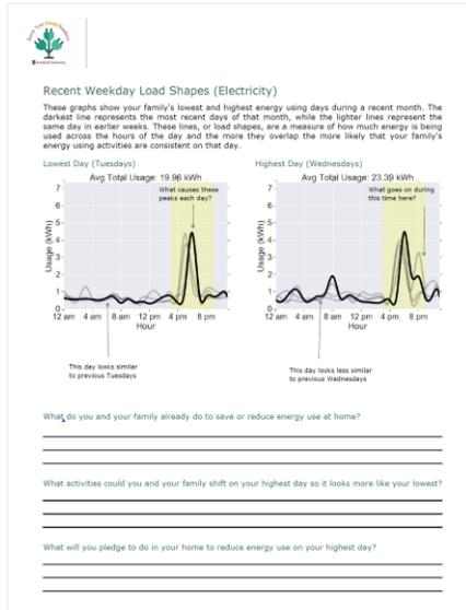
**Figure 4:** Using hourly smart meter energy data provided by parents, the research team designed and distributed a series of personalized energy visualizations that displayed daily, weekly, and yearly summaries of energy consumption. These handouts were designed to be engaging and included fill-in-the-blank type worksheets as well as personalized notes about household energy use.
