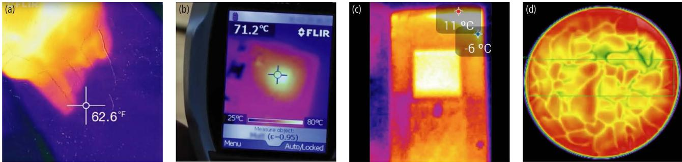
**Figure 3:** Illustrative examples described throughout our findings: (a) exploring whether thermal cameras can see through water in V90, (b) comparing a Raspberry Pi’s internal temperature sensor to a handheld thermal camera reading during a stress test in V801, (c) an exterior home inspection in V351, and (d) describing how convection in hot coffee causes cells to be visible in thermal images in V154.
