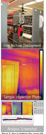
Figure 5: (top to bottom) Our sensor kit was placed in the center of the film archive, analysis was performed on large sections of walls and windows by the auditor, and the visualization tool provided views of the data.
