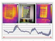
(b) By dragging the cursor along one the axes of PCP timeline, the user can filter by temperature and view corresponding spatial regions in the center image.
