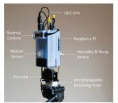
Figure 2: Prototype temporal thermography sensor kit used in the studies.
