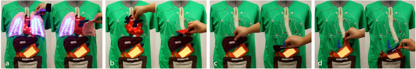
**Figure 6:** Using a conductive magnet approach, Prototype 3 allows for the dynamic removal and reattachment of the (a) lungs, (b) heart, (c) liver, and (d) part of the stomach enabling learners to explore the multiple organ layers of the human body. See supplementary video figure for more details.
