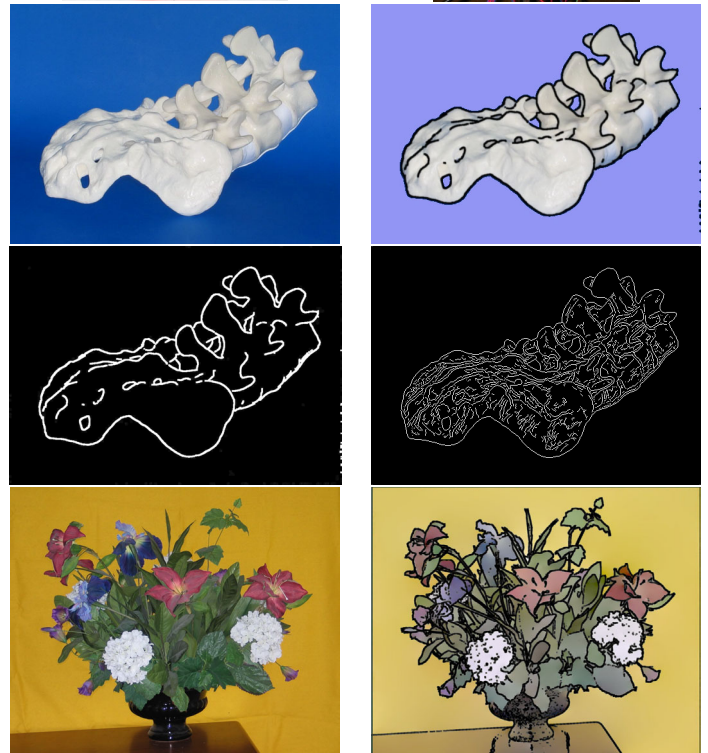
Figure 1. (Top row) The four-flash NPR camera prototype (Second) Source image, enhanced with depth edges (Third) Depth edges detected by NPR camera, compares with Canny edge detector (Fourth) Flower image, highlighted depth edges with de-emphasized texture.
