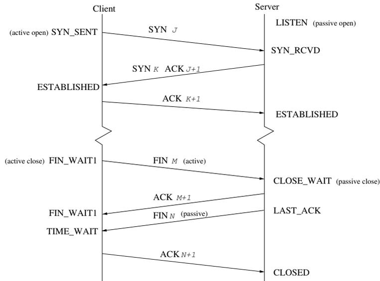
Figure 2: TCP states corresponding to normal connection establishment and teardown (from [54])
