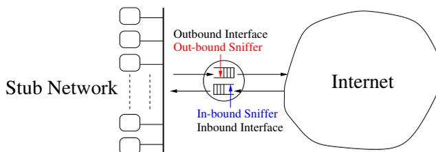
Figure 1: The structure of CPM placed at a leaf router
