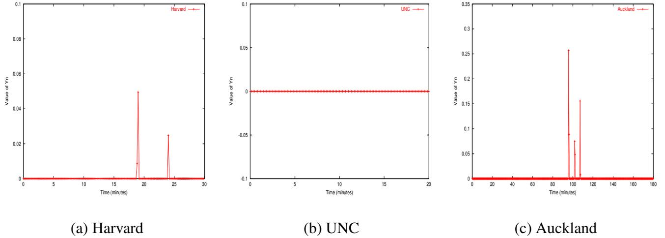
Figure 9: CUSUM test statistics under normal operation at: Harvard, UNC and Auckland
