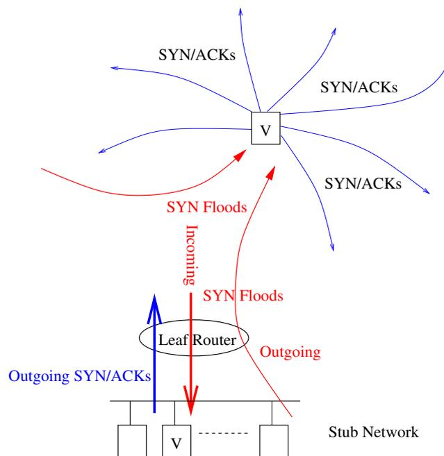
Figure 3: Match and mis-match between SYN vs. SYN/ACK pair at a leaf router
