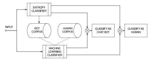
Figure 6: Classification System Diagram
