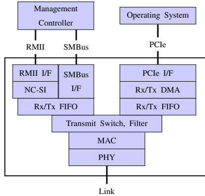
Fig. 3. Architecture Block Diagram of Intel 82574L [35]
