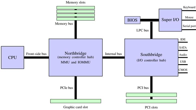
Fig. 2. Typical Hardware Layout of a Computer
