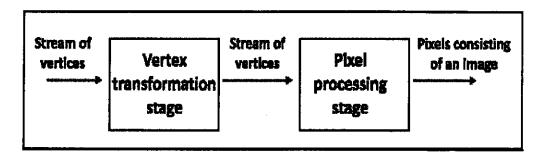
The traditional rendering pipeline has many stages. We can simplify those stages into two following two major steps: 1) vertex transformation stage (e.g., modeling and viewing transformation) step, and 2) pixel processing stage (e.g., rasterization). Since these two stages can be performed independently, we can perform these two stages in a parallel manner in graphics hardware.
