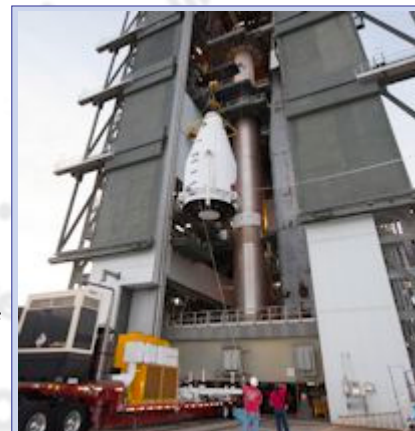
NASA's MAVEN spacecraft is hoisted to the top of an Atlas V rocket at Cape Canaveral. Launch is scheduled for Nov. 18th. Click for More
