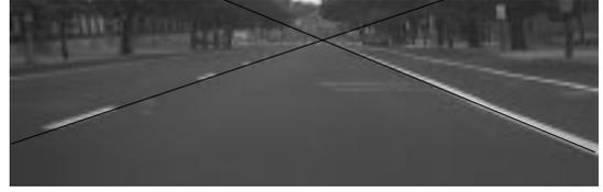
Figure 4. Extrinsic calibration. A road of known width, with lane marking lines marked by the user.
