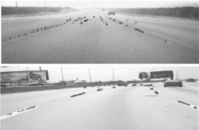
**Figure 5. Feature extraction examples (extracted features marked with black dots)**
