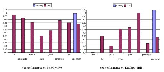
Figure 7. Optimizing scenario, Opt, tuned for Total execution time on x86 (Opt:Tot)
