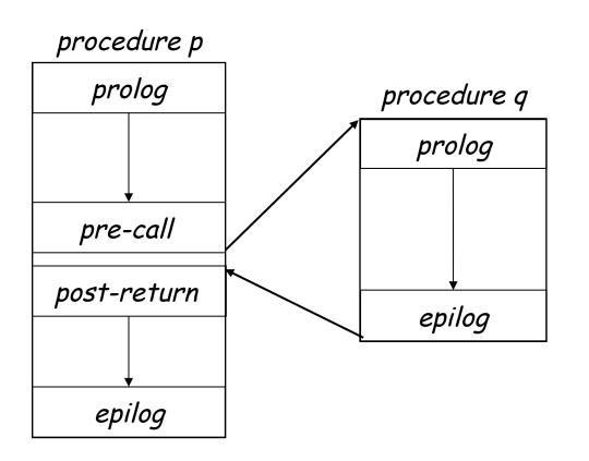
Procedure has • standard prolog • standard epilog Each call involves a • pre-call sequence • post-return sequence These are completely predictable from the call site ⇒ depend on the number & type of the actual parameters
