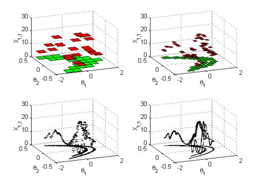
Figure 1: The above shows the 1-1 element of the quadratic cost of the optimal jump linear controller as the partition is refined. The cost converges to a continuous function which is the cost of the optimal LDV controller. For reference, the partition is shown in the z=0 plane.
