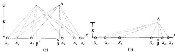
Figure 3. (a) The sample myriad,  $\hat{\beta}$ , minimizes the product of distances from point  $A$  to all samples. Any other value, such as  $x = \beta'$ , produces a higher product of distances; (b) the myriad as  $k$  is reduced.
