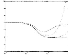
Figure 1. Values of the myriad as a function of  $k$  for the following data sets: (solid:)Original data set = 0, 1, 3, 6, 7, 8, 9; (dash-dot:)Original set plus an additional observation at 20; (dotted:)Additional observation at 100; (dashed:)Additional observations at 800, -500 and 700.
