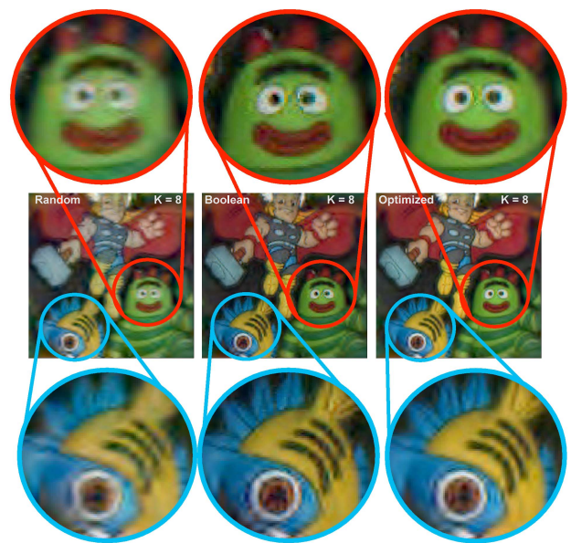
Fig. 7. Full data cube reconstructions when random, Boolean, and optimized patterned filter arrays are used, and K = 8 snapshots are captured. The 14-band data cubes are mapped to false-colored RGB profile to visually compare the color fidelity with the original target scene.
