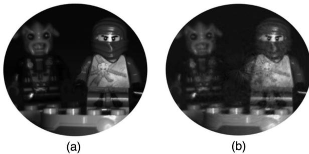
**Fig. 19.** (a) Original and (b) recovered images using the new coded aperture geometry with a rectangular sensor array.
