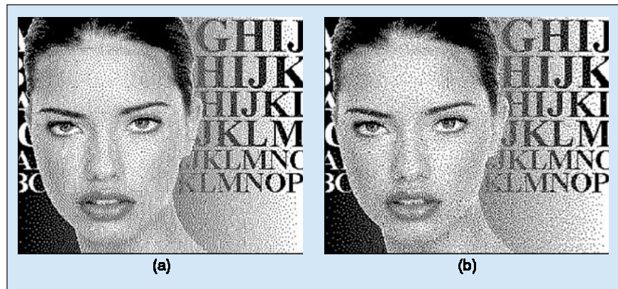
▲ 2. Grayscale images halftoned using (a) Floyd and Steinberg's original error diffusion algorithm and (b) Ulichney's perturbed filter weight scheme.
