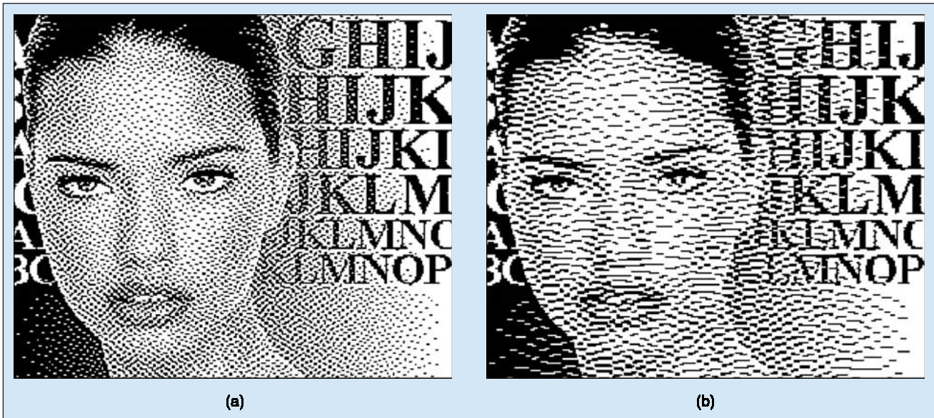
▲ 6. The image Adrian halftoned using Levien's error-diffusion with output-dependent feedback for hysteresis values (a) h = 1.0 and (b) h = 2.0 .
