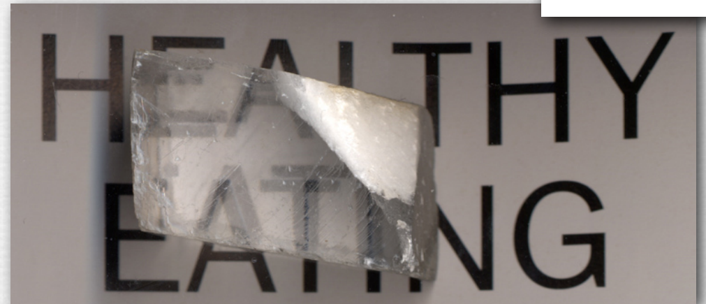
birefringence in a calcite crystal
