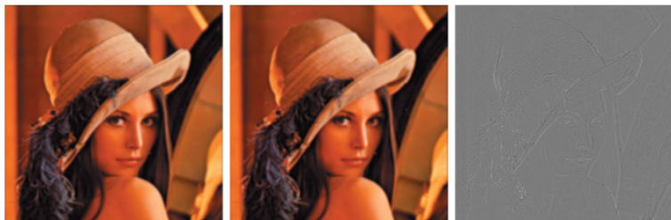
FIGURE 7.38 Image smoothing with a 5 \times 5 averaging kernel. (a) Result of processing each RGB component image. (b) Result of processing the intensity component of the HSI image and converting to RGB. (c) Difference between the two results.
