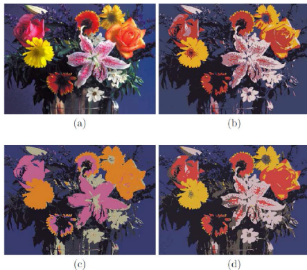
Figure 5.7 (a) Original color image. Results of segmentation using the k -means clustering algorithm in three different color spaces: (b) sRGB , (c) HSV , and (d) L^*a^*b^* . In each case, the image has been segmented into six regions. The color assigned to each region is the final centroid of the color values in the corresponding region in the original image after application of the k -means algorithm.
