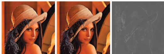
FIGURE 7.39 Image sharpening using the Laplacian. (a) Result of processing each RGB channel. (b) Result of processing the HSI intensity component and converting to RGB. (c) Difference between the two results.
